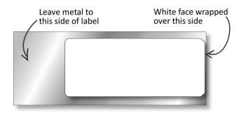
Smallest recommended bending diameter of the Confidex Silverline Blade II<sup>™</sup> is 100mm. For optimal performance please bend the label in the orientation shown below.
